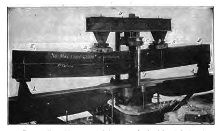
Fig. 32.—View of beam at completion of test showing failure in horizontal shear. Note that beam has split along center so that top half projects above lower half at end. AA, support for beam on weighing platform. BB, points where load is applied. C, head of screw press. D, straining beam. EE, fine wire stretched along center of beam. F, scale used with wire for measuring deflection of beam under load.
